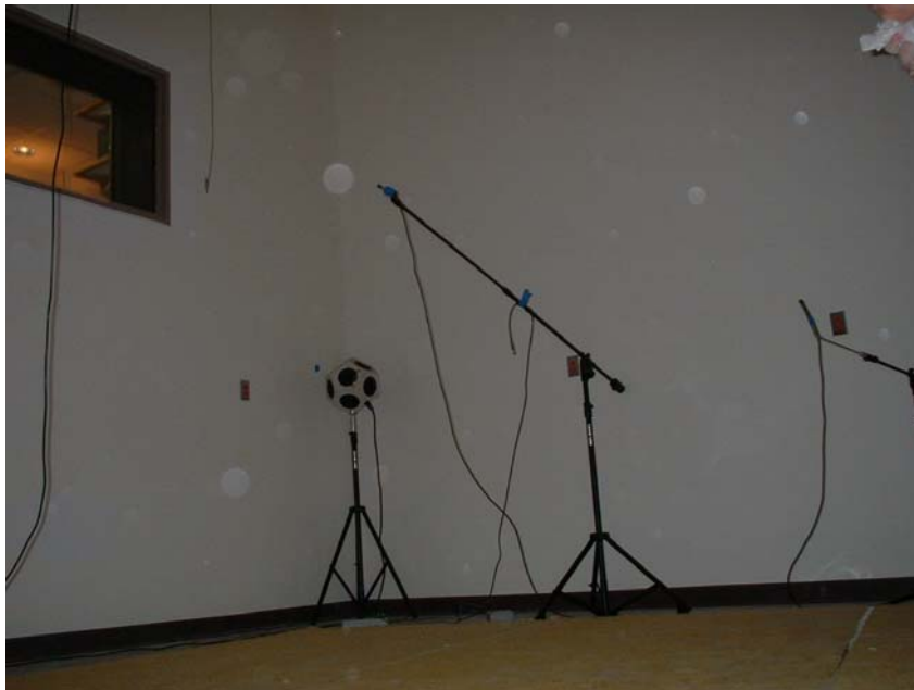
FIG. 2.4. Dodecahedron sound source.
